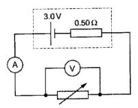
The reading on the ammeter I and the reading on the voltmeter V are recorded.
