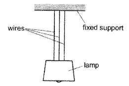
The weight of the lamp causes each wire to have an extension of 0.40 cm. The height h of the lamp above the floor is measured.
