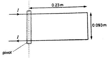
The U-shaped wire experiences a turning moment about the pivot of value 7.4 x 10<sup>-3</sup> N m.
