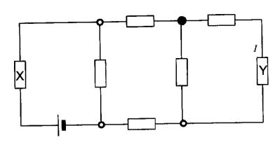
If the current in resistor Y is I, what is the current in resistor X?
