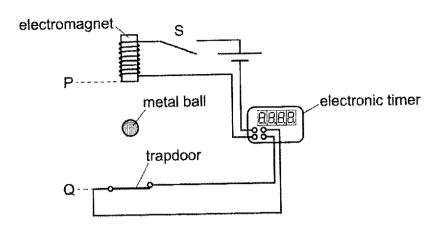
When switch S is opened, the ball is released from an electromagnet and an electronic timer is started. The ball then falls vertically downwards. The timer stops when the ball hits a trapdoor. The student measures the distance PQ between the electromagnet and the trapdoor. This distance and the reading on the timer are then used to calculate the acceleration of free fall.
