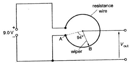
A wiper (variable terminal) can rotate and make contact with any part of the resistance wire.
