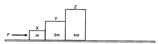
What is the ratio  $\frac{\text{force exerted on block X by block Y}}{\text{force on block Y by block Z}}$ ?
