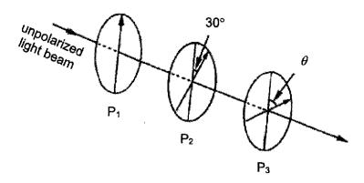
The polarised light beam incident on  $P_2$  has an intensity of 30 W m<sup>-2</sup> while the light beam emerging from  $P_3$  has an intensity of 14 W m<sup>-2</sup>.
