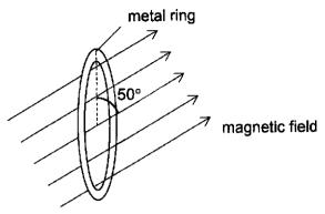
The magnetic flux density through the ring decreases by  $4.0 \times 10^{-5}$  T at a constant rate in 2.0 s. During this change, what is the current induced in the ring?
