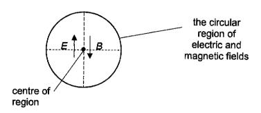
The deflections of the beam from the centre of the region produced by the electric field E and the magnetic field B acting separately are equal in magnitude.
