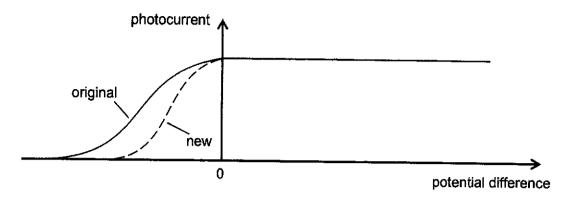
The light source is then replaced with a new one, and the dashed curve is obtained.
