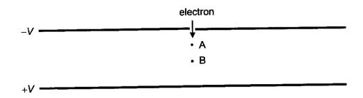
The two plates are at electric potentials -V and +V.
