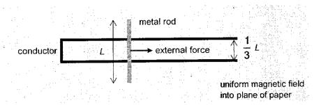
The two parallel sections are separated by  $\frac{1}{3}L$ . An external force causes the metal rod to slide at constant speed v.
