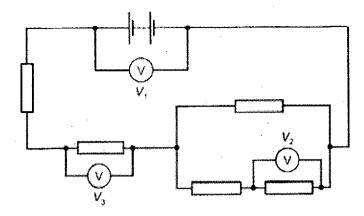
The reading  $V_1$  is 8.0 V and the reading  $V_2$  is 1.0 V.
