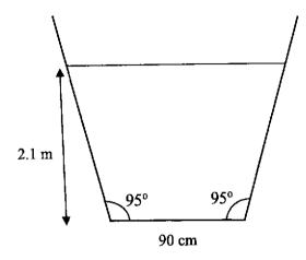
(a) Calculate the volume of water in the canal.
