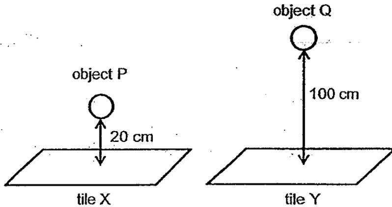
2 identical tiles were placed on the floor just below each object. Tile Y broke when object Q landed on it but tile X did not break when object P landed on it.
