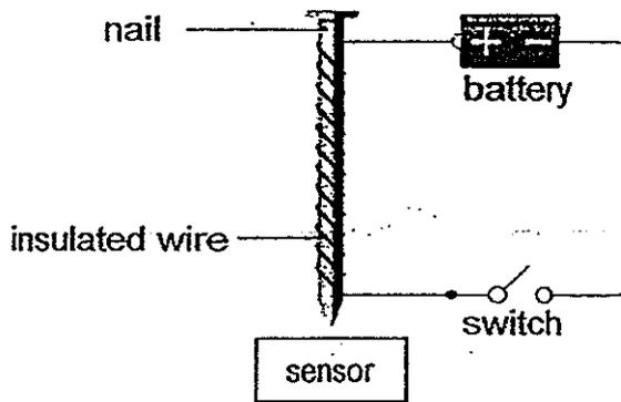
He used a sensor to measure the strength of the electromagnet. He placed the sensor 3 cm from the magnet and increased the number of batteries. He repeated the experiment with the sensor 5 cm from the electromagnet.
