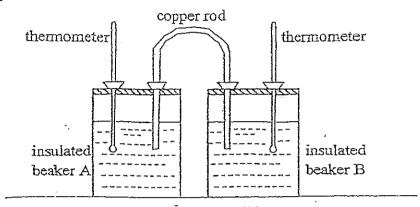
She connected a copper rod to two insulated beakers containing equal amounts of the same type of liquid. The temperature of the liquid in Beaker A was 95°C and the temperature of the liquid in Beaker B was 5°C.
