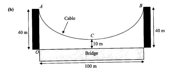
The diagram shows a horizontal bridge of 100 metres supported by 2 pillars at the side, with a cable being suspended from point A and B. Each pillar is vertical and is 40 metres tall. The lowest point C of the cable is 10 meters above the bridge. The origin, O, is vertically below point A, where the foot of the pillar meets the bridge.
