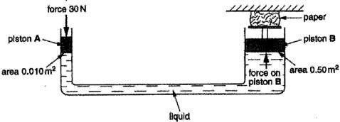
A force of 30 N applied at piston **A** exerts a pressure. The liquid transmits this pressure to piston **B** which then causes a force to be exerted on the paper.
