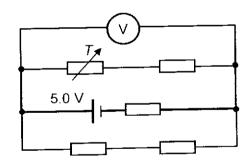
The resistance of each resistor is 1.0 k $\Omega$  and the resistance of  ${\cal T}$  is 5.0 k $\Omega$ . What is the reading of the ideal voltmeter?
